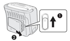
3 Install the battery pack in the printer.
